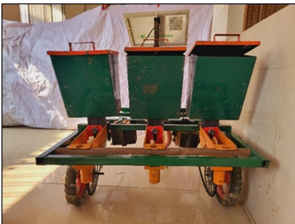
Fig 3: Back view of machine including seed metering mechanism
