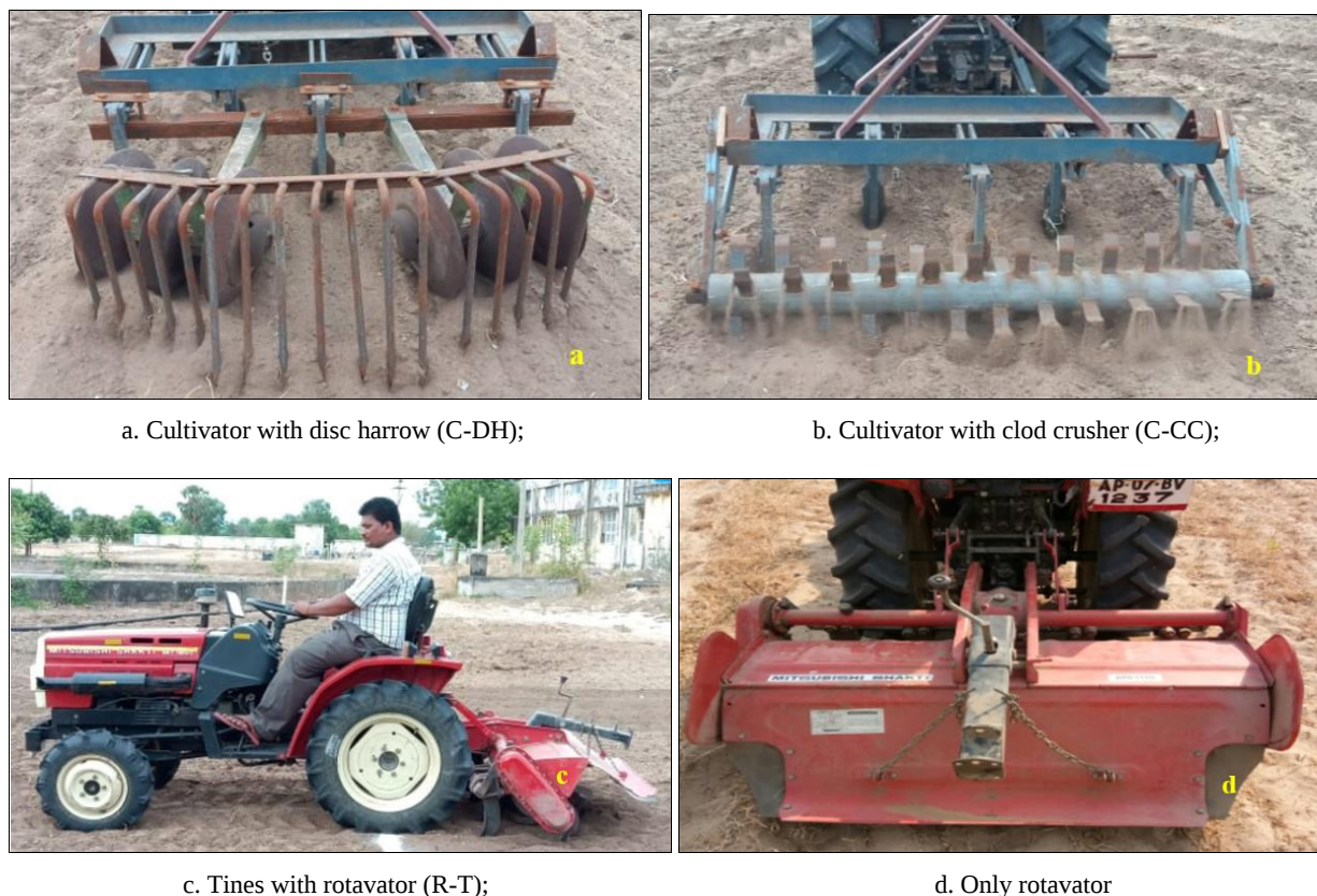
Fig 2.1: Developed combination tillage implements with test tractor
