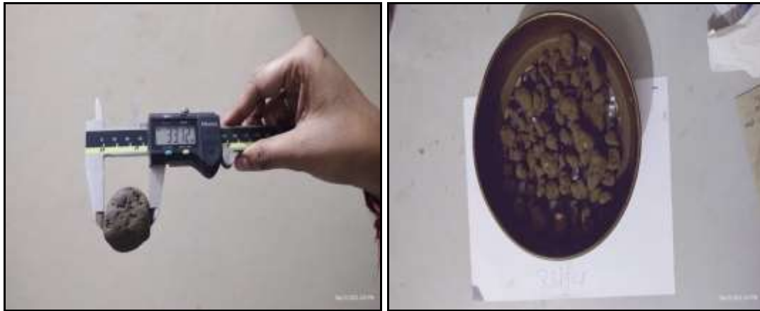
Plate 2: Measuring the mean weight diameter of the soil sample
