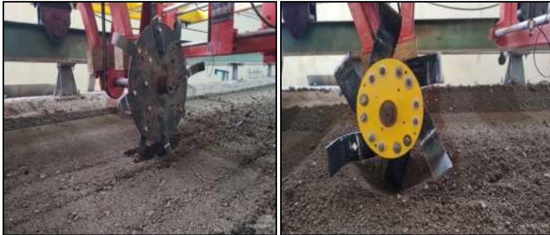
Plate 1: L and J-shaped rotary blade during test under soil bin
