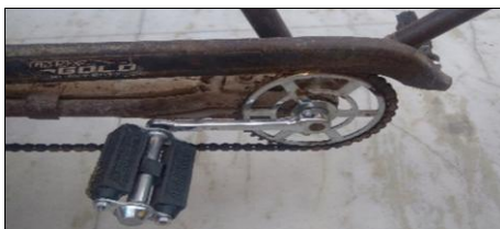
Plate 11: Modified Chain Drive Gear (Number of teeth reduced from 43 to 31)
