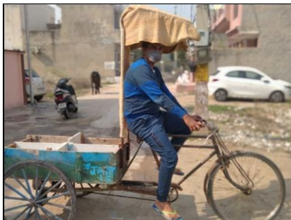
Plate 1, 2 & 3: Pictures of Roof shade/Canopy in Modified Loading Rickshaw (GSLR)
