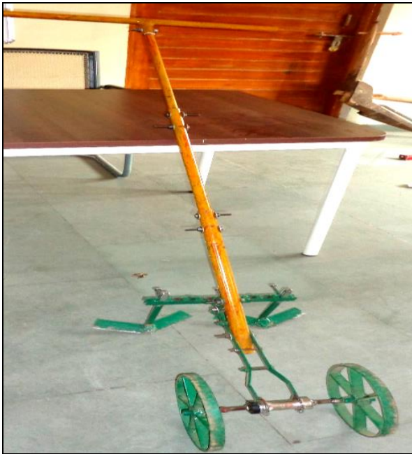
Fig 2: Manually operated twin wheel weeder with adjustable blades
