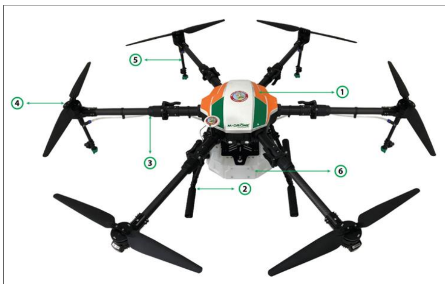
Fig 4: MD-10H Agri Drone, 1. Centre body; 2. Landing gear; 3. Arm set; 4. BLDC Motor with propeller; 5. T-Jet nozzle; 6. Agricultural tank
