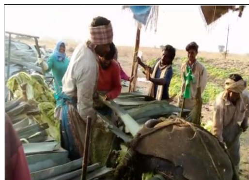
Fig 2: Mechanical decortication of Agave using raspador machine
